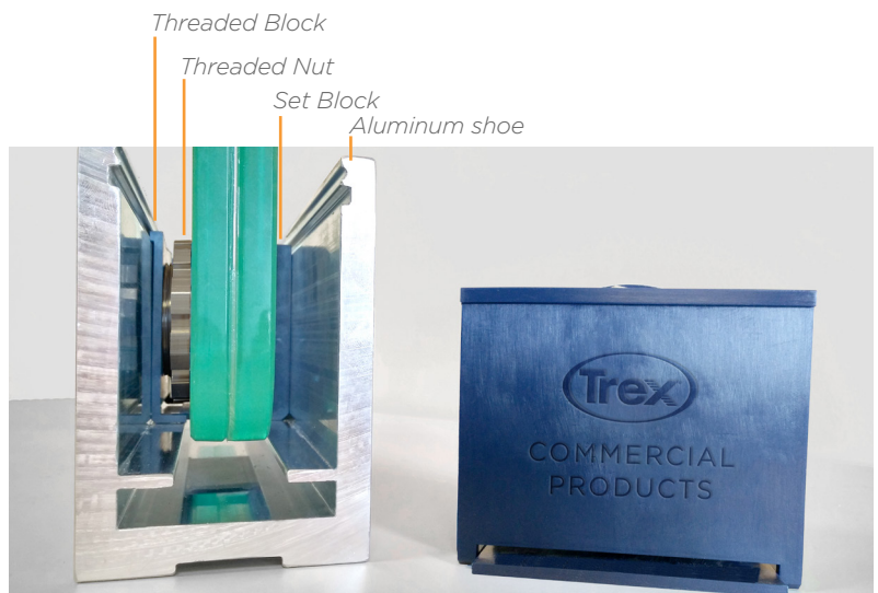
Clear half-inch glass is secured within an aluminum shoe using Trex Commercial Products' dry glaze GlassNut™ Track Rail system, with a black gasket finishing off the look.
